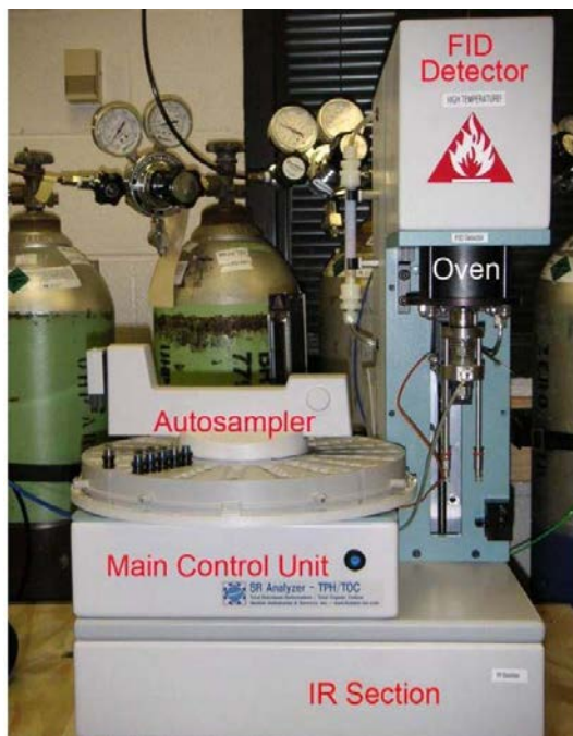
Figure 1. Four Main Components of the SRA System.
