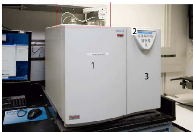
Figure 1. Elemental Analyzer: (1) Furnace Access Door, (2) Synoptic Panel, and (3) Thermostatic Chamber Access. Dry Sample Autosampler is located on top of furnace.
