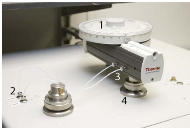
Figure 2. Dry Sample Autosampler (red box in Figure 1): (1) Drum, (2) Gas Connection Fitting, (3) Gas Tube, and (4) Reactor Fitting..
