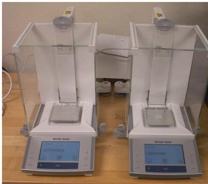
Figure 1. Mettler-Toledo XS204 Dual Analytical Balance System.
