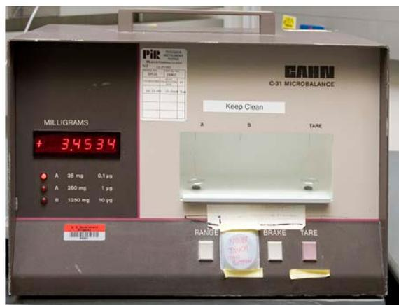
Figure 2. Cahn C31 Electrobalance.
