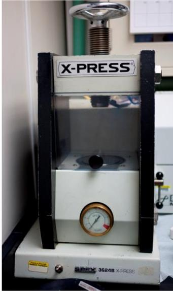
Figure 2. X-Press Sample Crusher.
