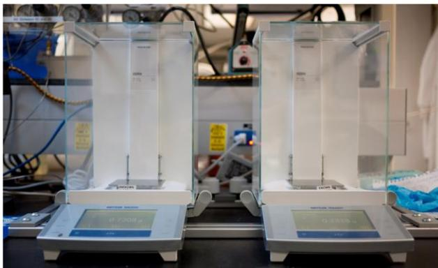
Figure 1. Mettler-Toledo Dual Analytical Balance System.
