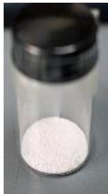
Figure 9. Prewighed Vial Containing Lithium Metaborate Flux.
