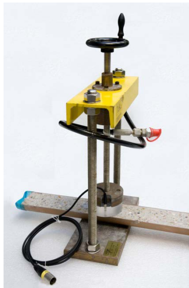
Figure 2. Thermal conductivity measurement on hard rock sample using half-space puck.
