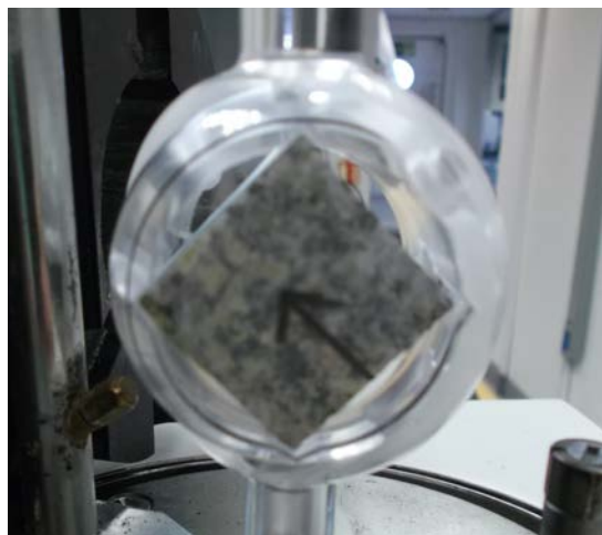
Figure 8: Hard rock sample in automatic holder of spinner.
