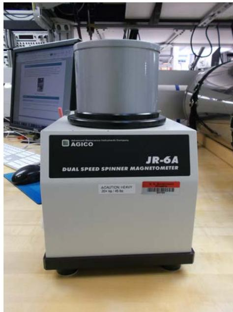
**Figure 1:** JR-6A in the Paleomagnetism Lab.
