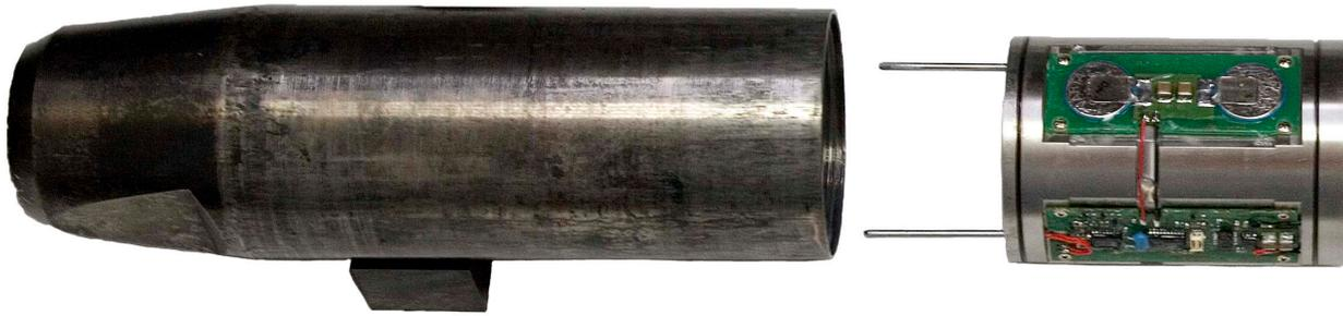
**APCT-3 shoe (left) has a pocket to accept electronics, memory board, and battery (right) for temperature measurements while taking an APC core.**
