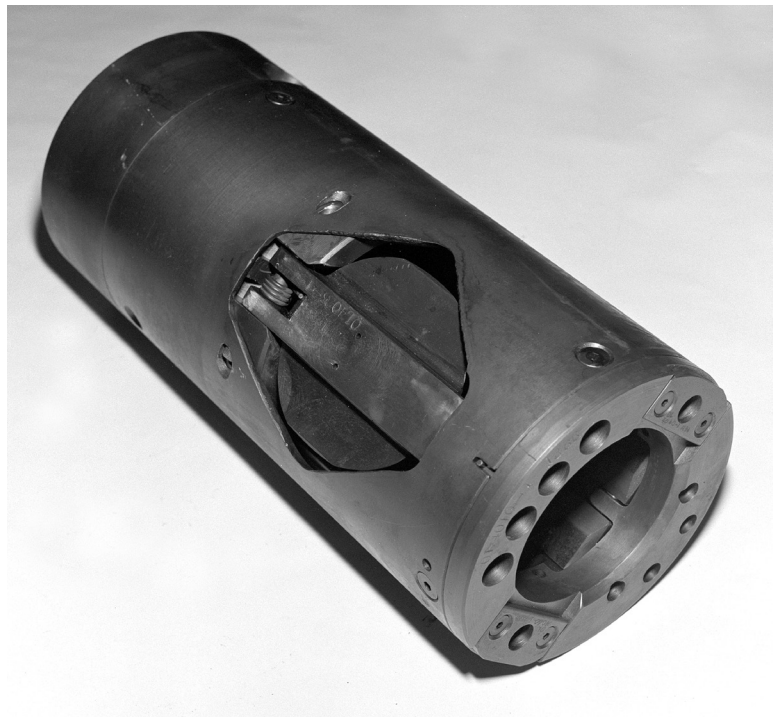
The LFV showing the flapper in the locked-open position.
