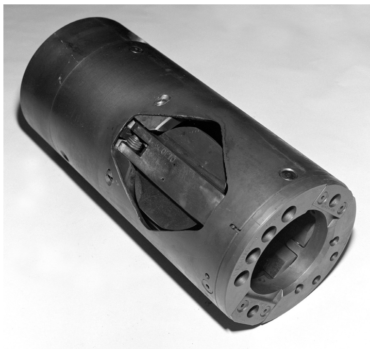
The LFV showing the flapper in the locked-open position.
