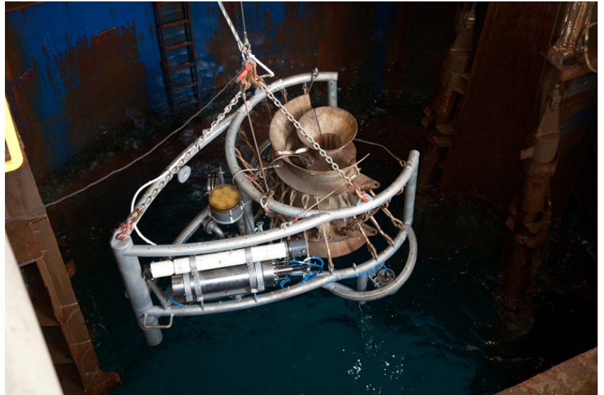
VIT being deployed in the moonpool.
