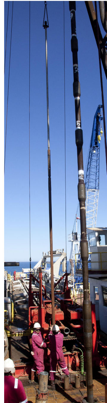
Half-Length APC being deployed on the rig floor.
