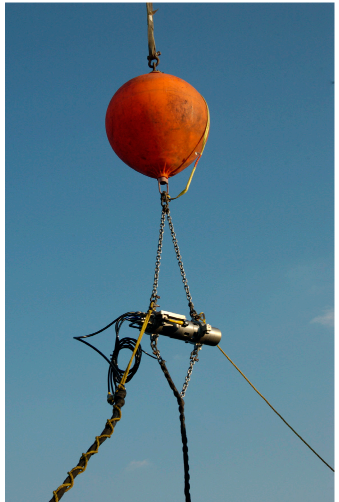
Air gun being lifted by one of the ship's cranes.
